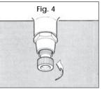
3. Before transporting your compressor or when leaving overnight, expel all air from the receiver by opening drain valve (Fig.4).
