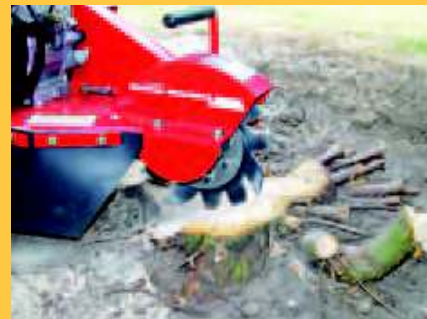
Tungsten Tipped Blade in Action
