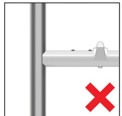
Diagonal braces **must** always be located with the claw opening facing down. Horizontal braces must be located with the claw facing either down (on the rung) or outwards (if on the upright).
